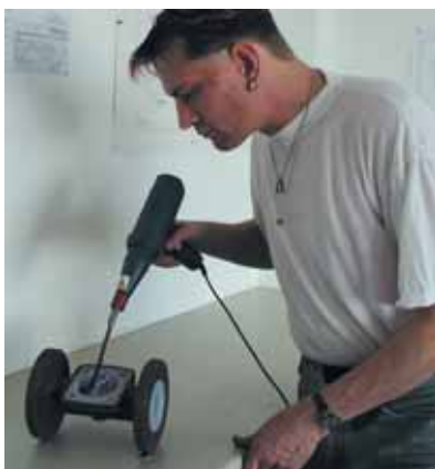
High frequency spark testing of body lining
