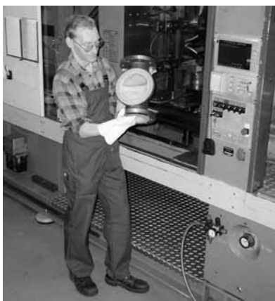
Injection moulding machine during production of lined diaphragm valve bodies.
