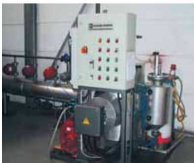
Test stand for continuous improvement with saturated steam up to 230 °C / 450 °F
